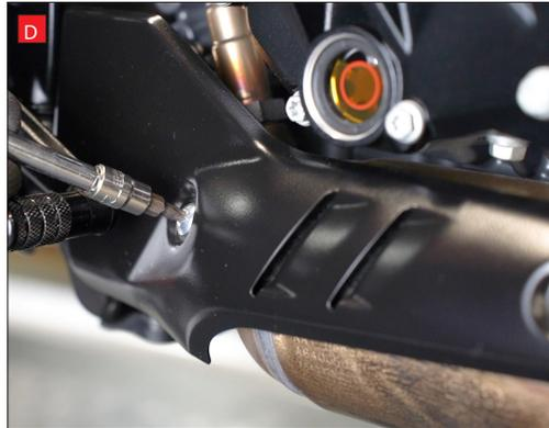
D) Remove the heat shield from the catalyst.
