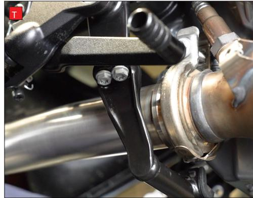
W) Refit the heat shield to the cat.
