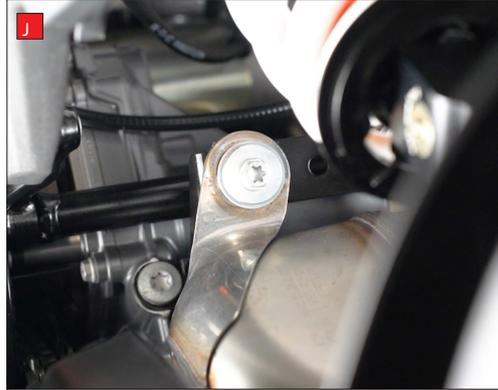
I) Remove the clamp between the cat and the centre silencer.
