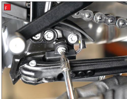
H) On the right hand side of the bike remove the 2 bolts for the side stand frame, then remove the frame from the bike.
