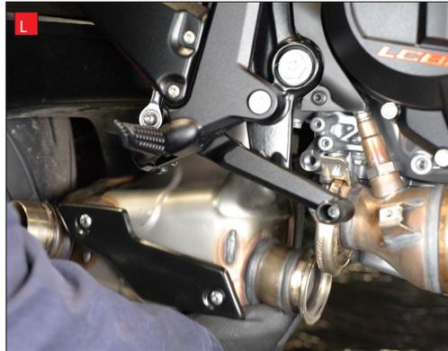
N) Put the Scorpion Silencer Delete Pipe in position and loosely secure in place with the original clamp, you will fully tighten in a later step. Ensure that the tab on the clamp is aligned with the notch on the pipe.
