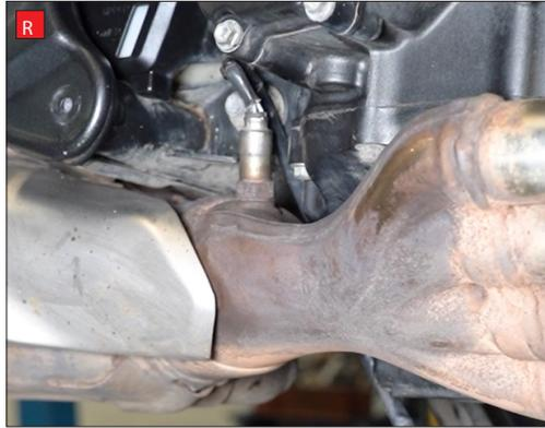
Q) On the left hand side of the bike, remove the Lambda sensor from the exhaust.
