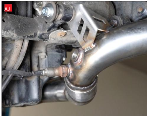
AJ) Screw the front Lambda sensor into the front boss. Fully tighten.
