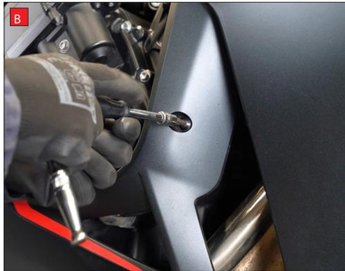
A) On the right hand side of the bike remove the bolt from the rear of the fairing.
