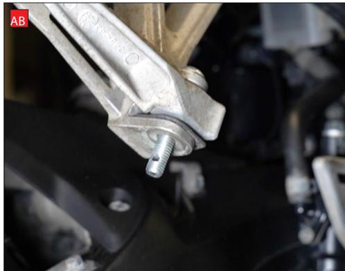
AC) Screw the bracket on but don't fully tighten yet, you will do that in a later step.
