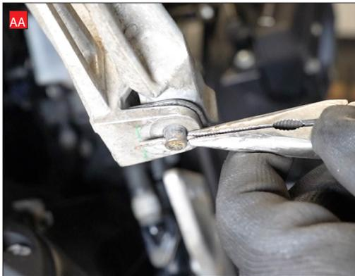
AB) Remove the spindle and replace it with the drilled bolt supplied in the kit.
