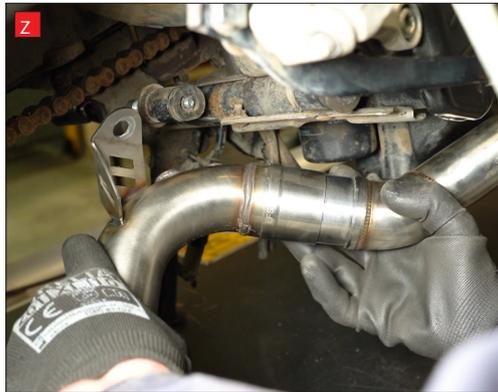
Z) Slide the Scorpion connecting pipe onto the collector.
