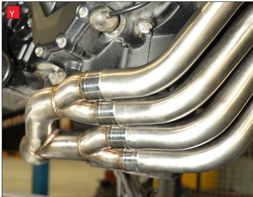
Y) Slide the collector onto the header pipes.
