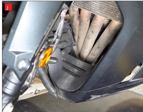
I) On both sides of the bike, remove the fixings that hold the inner plastic panel to the fairing.
