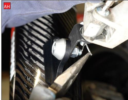
AH) Fully tighten the rear footpeg bolt. Do not over tighten as that will prevent the footpeg from opening and closing. Then insert the split pin into the hole and bend the ends.
