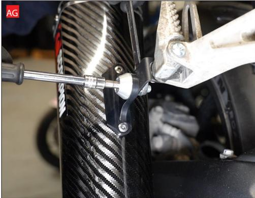
AG) Fully tighten the silencer mounting bolt.
