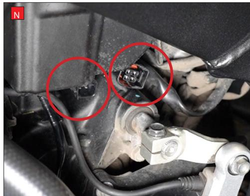
P) Release the 2 clips holding the Lambda sensor cables to the bracket just to the side of the oil filter.
