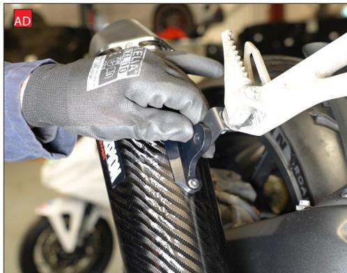
AE) Fit the springs between the spring hoops on the silencer and connecting pipe.
