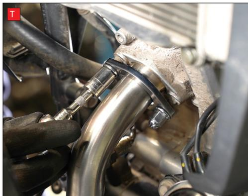
T) Adjust the system if necessary, then fully tighten the header nuts.
