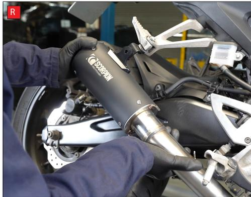
Q) Slide the Scorpion connecting pipe with the clamp onto the header pipe.
