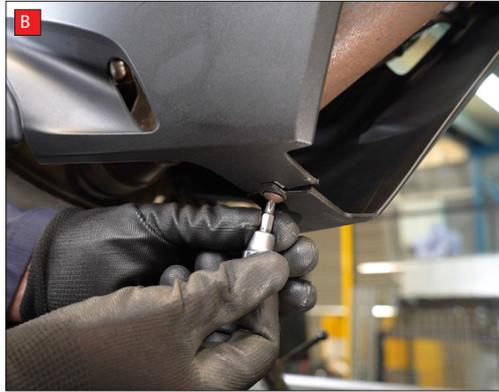
A) On the right hand side of the bike, remove the bolt from the back of the lower fairing.
